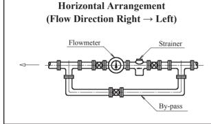
• As shown below, install a strainer at the up-stream of the flowmeter and provide a by-pass for the convenience of flowmeter disassembly and maintenance.
